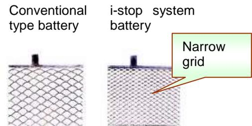
(2) Charging ability is improved by reducing **sulfation** due to discharging.
