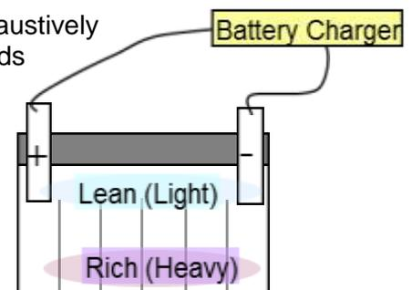
② **Inspection by voltage/specific gravity measurement**
